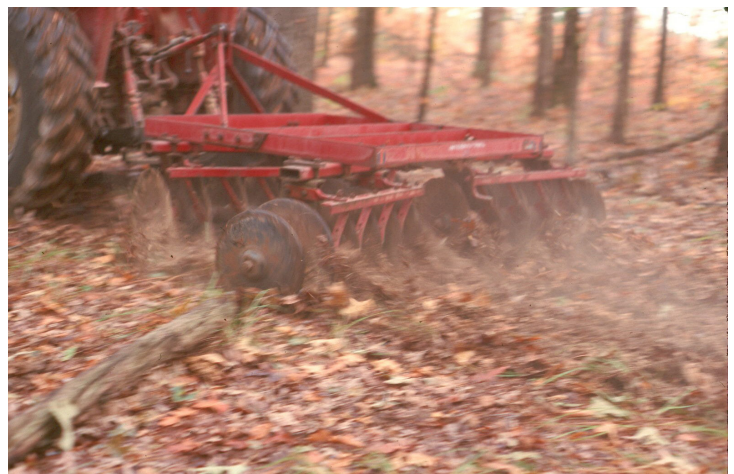
Figure 2. Disk scarification operation in a bottomland oak stand.
