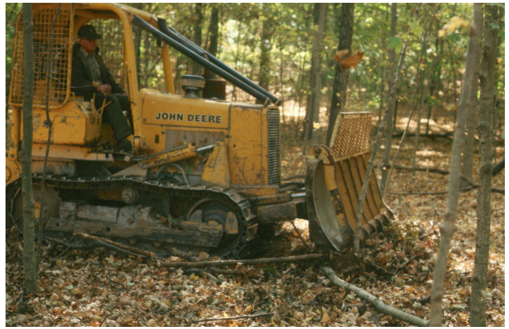
Figure 1. Brushrake scarification conducted in a mature upland oak stand.
