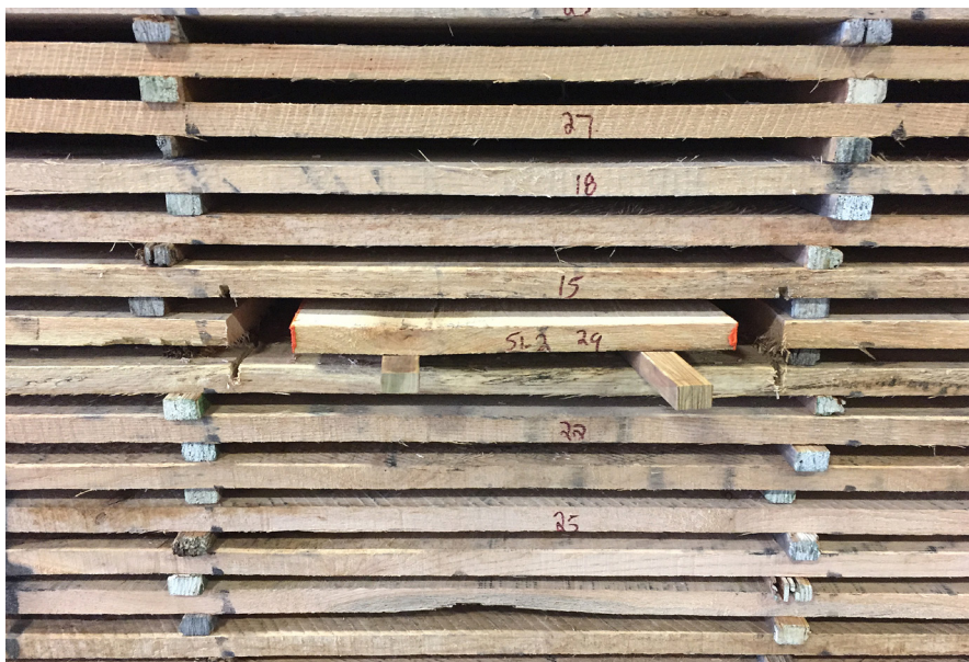
Figure 3. One way to label sample boards and insert them into a stack of lumber. The stickers shown here are spaced two feet apart for 4/4 lumber. Note the Bright Orange Sample Sealer (B.O.S.S.) used by this firm to coat the ends of their sample boards. (B.O.S.S. is sold by Anchorseal.)
