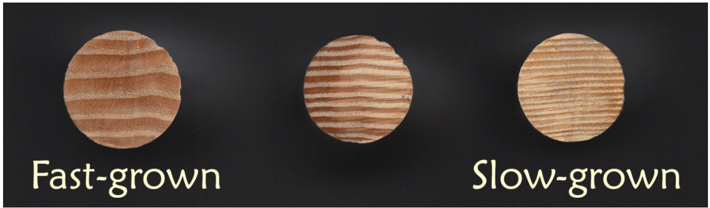
Figure 2-7. White ash cross-sections, fast- to slow-grown. The fast-grown samples have significantly wider growth rings; the lighter-colored wood is the earlywood and the darker wood is the latewood.
