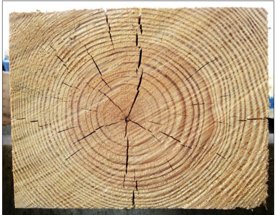
Figure 2-9. This railroad tie is made from southern pine. The center of the tree has wide growth rings, indicating that the growing conditions were probably uncrowded for the first few years after the tree was planted. After about eight years or so, the adjoining tree canopies began to close in and the overall growth started to slow down (as indicated by the narrower growth rings). Notice the pumpkin-colored heartwood surrounding pencil-sized pith in the center of the tree.
