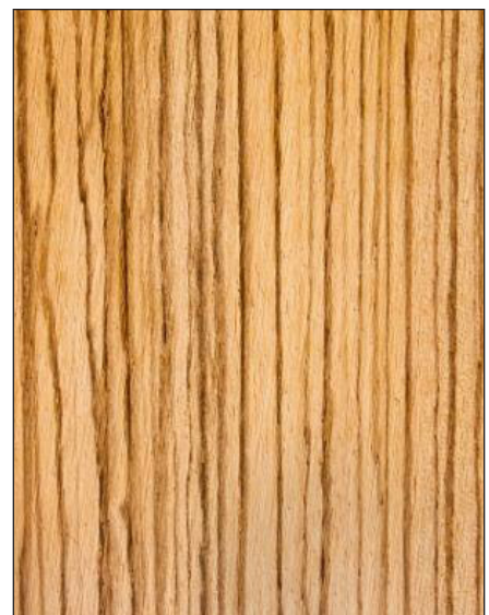
Figure 2-3. Zebrawood ( Microberlinia spp.) is so named because of its distinctive dark-and-light striped pattern.
